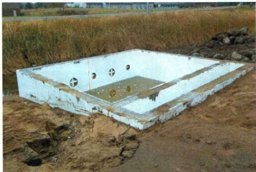
In the spring of 2014, a new storm water application will be tested in Aitkin, Minn., for the removal of copper from the storm water running off a grocery store parking lot.
