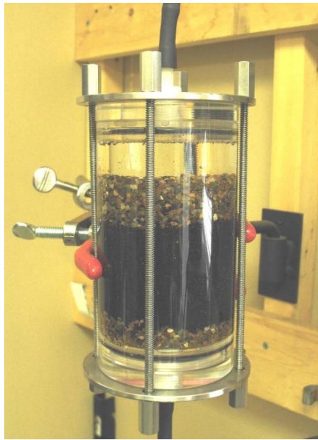
Bench scale treatment column of APTsorb
